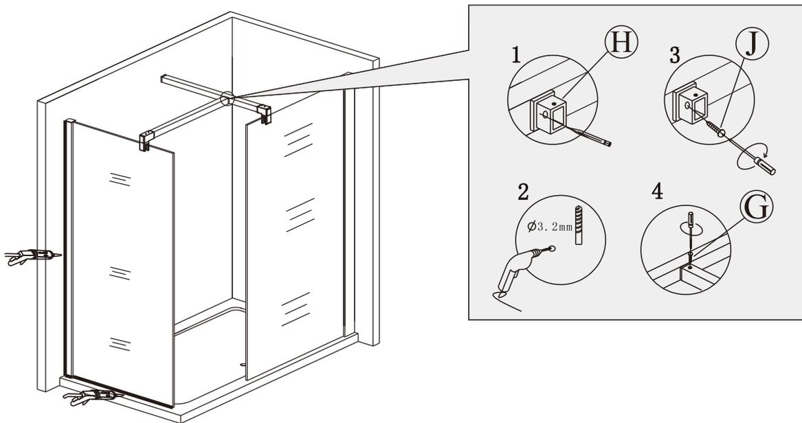
Apply some silicone on the outside edge of the shower enclosure (between the wall profiles and wall and between the frame and the tray) to enhance waterproof. After installation, it needs 24hours for silicone to dry before being put into use.
